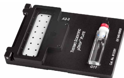
Figure 1. μDrop Plate. A low sample volume measurement area with 16 measurement locations on the left and a cuvette location for a 10 mm cuvette on the right.
